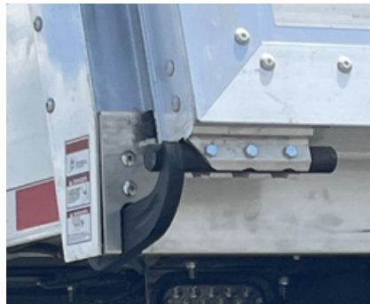
Rotating tailgate lock pin.
