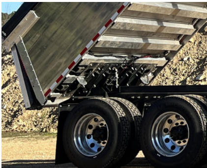
3" diameter steel rear body hinge for extended wear.
