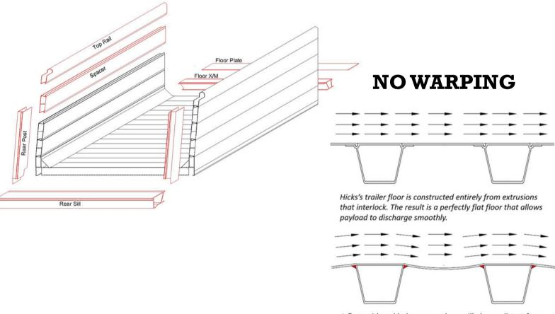
A floor with welded crossmembers will always distort from heat. The result is a "washboard" surface with high spots that will wear excessively with discharge payload.
